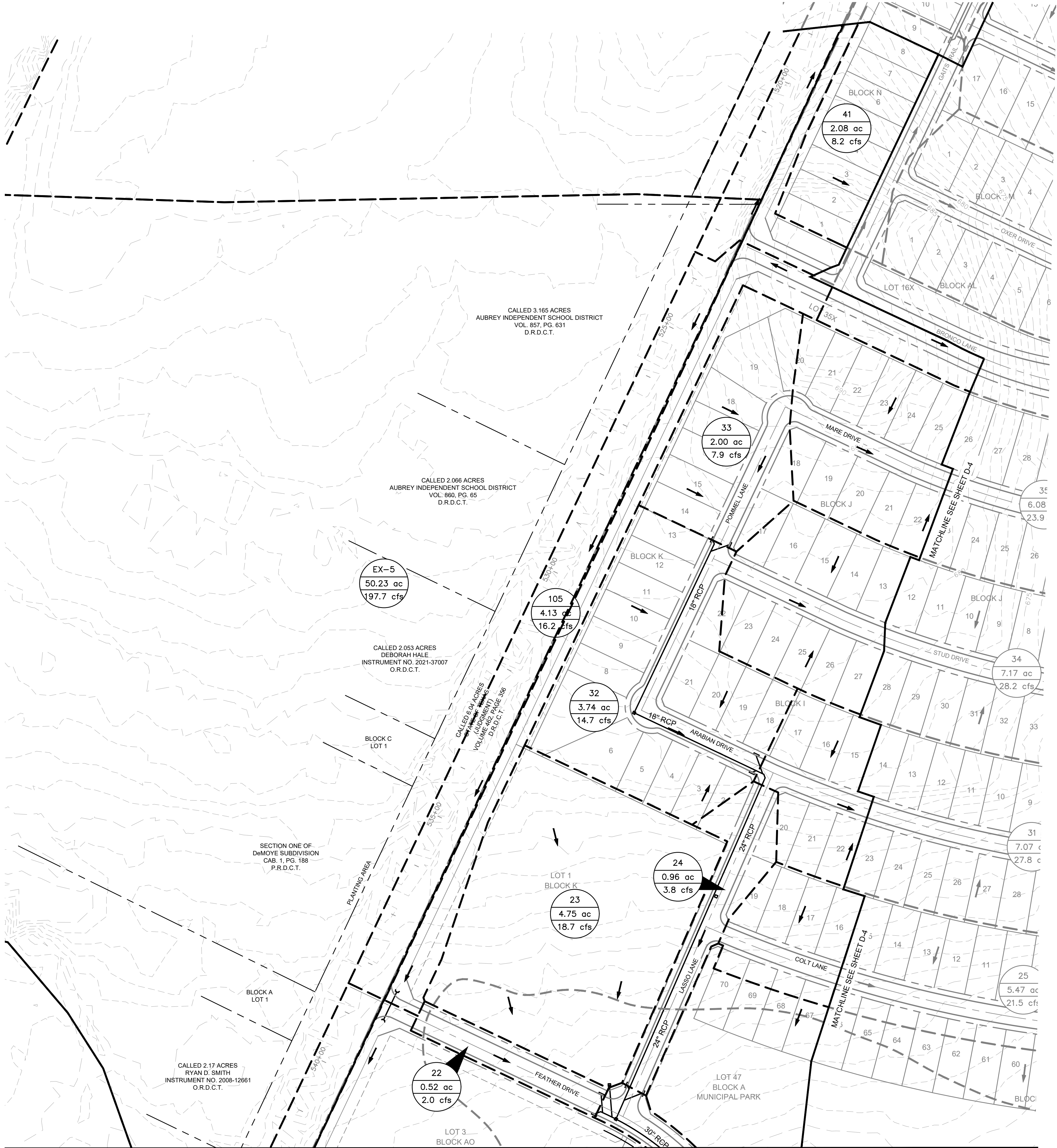
LOT GRADING TYPE B DRAINAGE BOTH TO STREET & REAR LOT LINE
